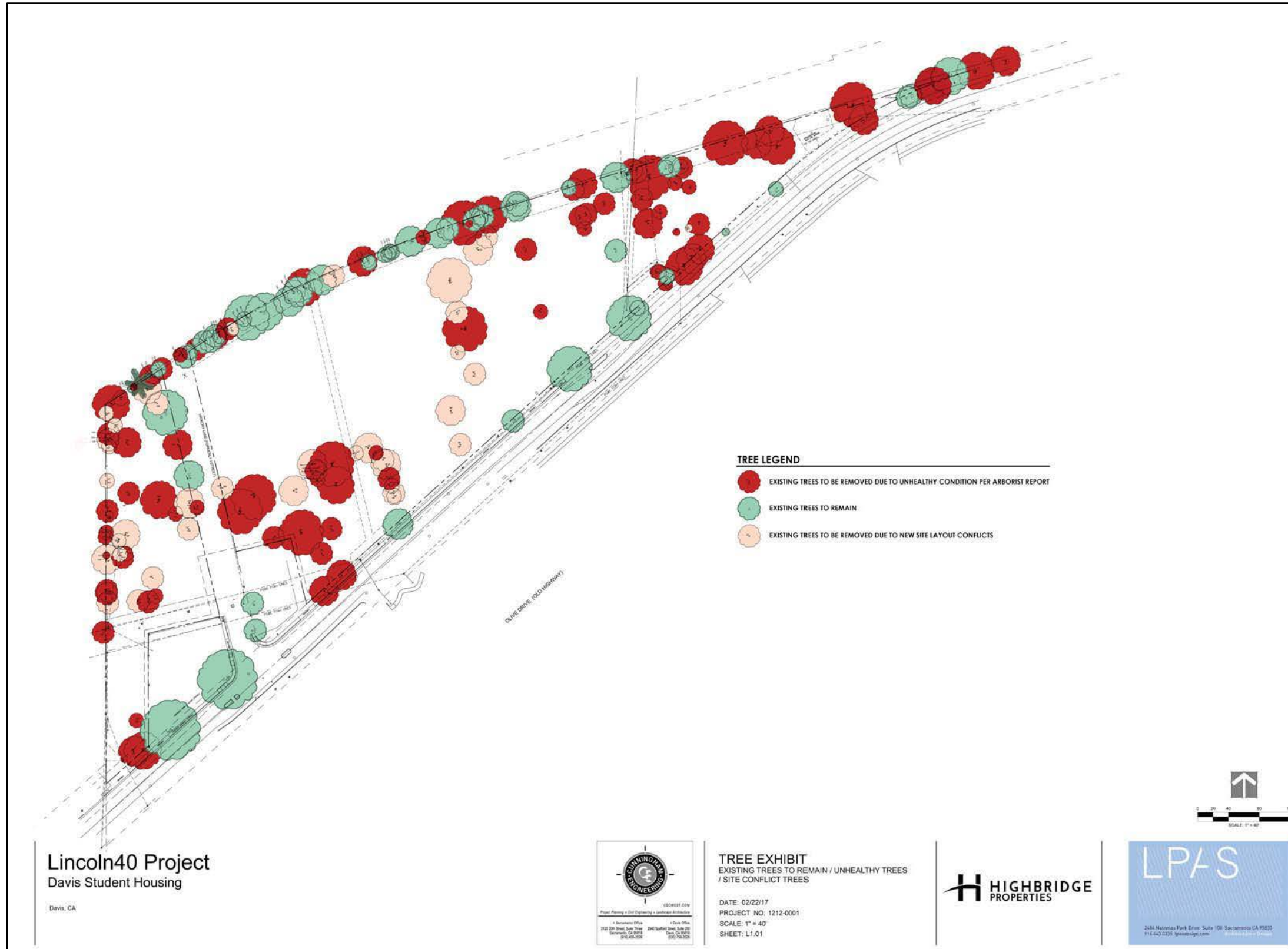
Figure 3-8 Trees to be Removed and Retained
