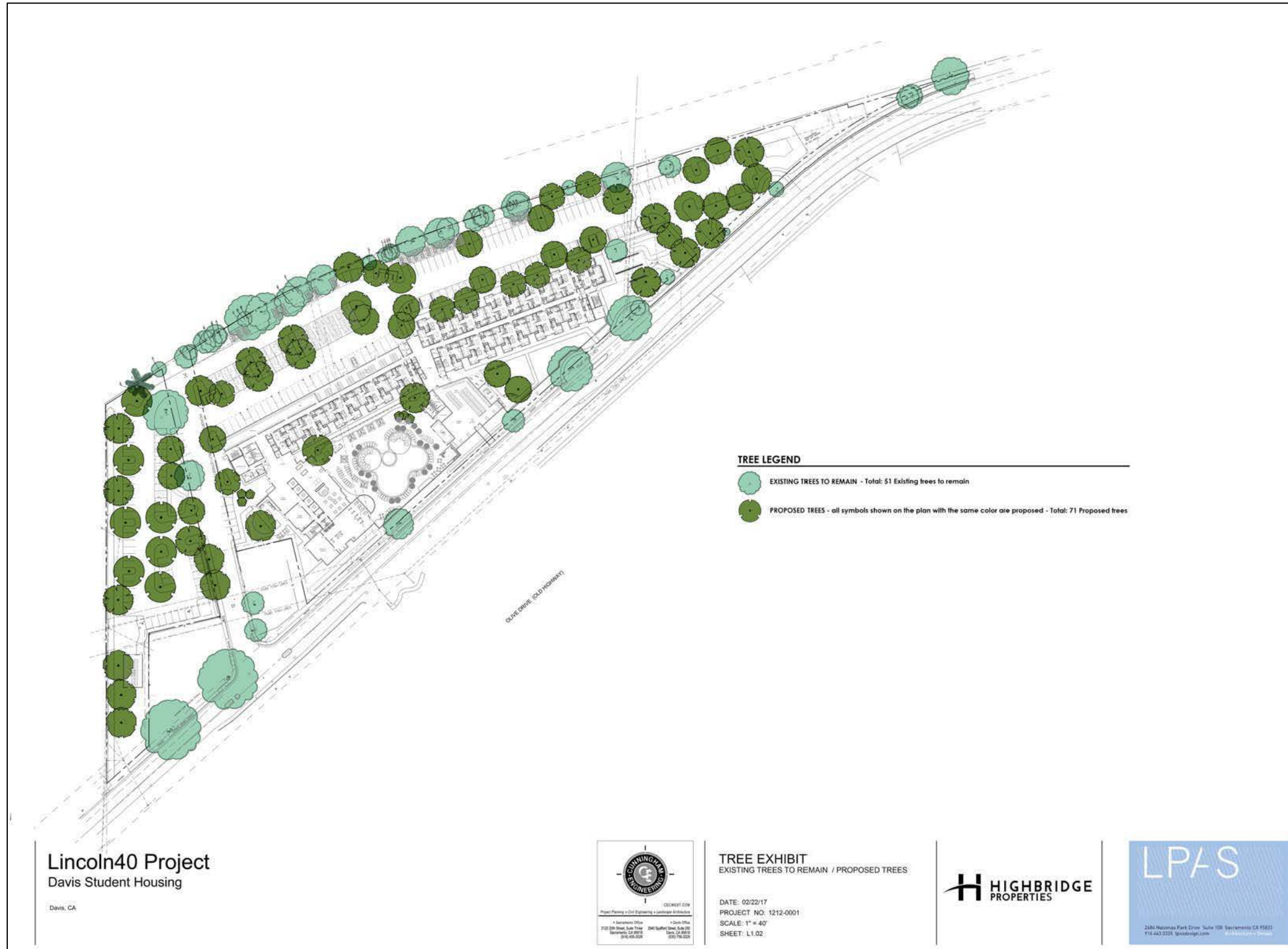
Figure 3-9 Trees to be Retained and Planted
